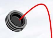
Snap metal housing with processing insert on top of the blockout ring on the abutment
